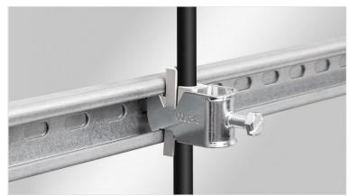
The cable clamps are characterised by a high clamping range and great flexibility. Ideally suited for strain relief on the C section rail with opening dimensions 16 - 17 mm. It offers flexible clamping ranges from 6 mm to 64 mm. The counter tray is secured by a locking mechanism and cannot slip out of the cable clamp.
