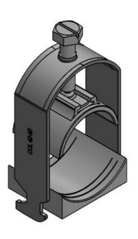
Part No. 32006 Clamping 1 x 42 - 50 EAN **4251269323** range mm 638 Package 25 quantity Length 24 mm Width 55 mm 83 mm Height Mounting 101 mm height
